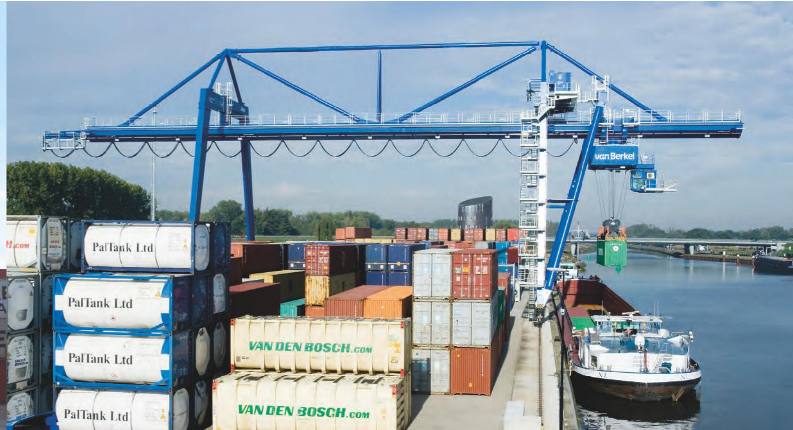
Kuenz Barge Crane with aerodynamic girder at the Van Berkel Logistics Terminal
